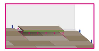
7b. Place another plank on top of that board making sure it touches the wall
