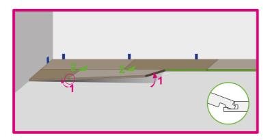
5: in order to complete the installation, you will need to push the planks to the floor to lock them
