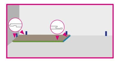
2. Place the second plank by inserting it in the groove (in blue in the drawing) of the  $1^{st}$  plank. Be careful not to damage the corners of the planks.
