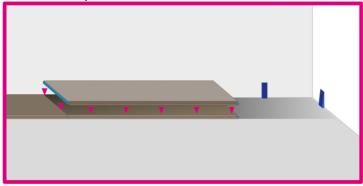
3b. Place another plank on top of that board making sure it touches the wall
