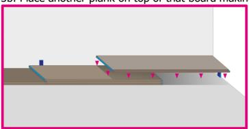
3c. Trace a line with a pencil on the former plank: this is the plank which will be cut and installed to finish the line
