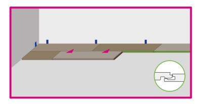
4c: Insert the tongues of the second plank in the groove of the plank of the first row. You will need to raise slightly the first plank to do so
