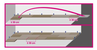
**Caution:** once you have installed the 1<sup>st</sup> plank of the second row, you should assemble the following planks by always starting with their short end tongue (in blue in the drawing). Before inserting the plank in the long side groove (in green in the drawing), slightly raise both planks before pushing them down together. Follow the next steps:
