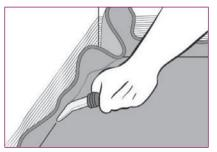
When coving, use a Tarkett Hockey Stick (art. no. 1258003) or similar tool to press the material firmly into the juncture between the floor and wall.
