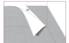
The corner seam shall be placed on one of the walls at a 45-degree angle.
