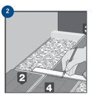
Turn the next board so it lies tongue to tongue with the first. Slide it along until the end is flush against the wall. Mark a cutting line 8-10 mm (must be the same size as the expansion gap) from the end. Cut the board with a handsaw. Slide the board into place and insert a spacer at the end. If a hand saw is used, saw from the top face of the board. If a circular saw or keyhole saw is used, turn the board and saw from the underside.
