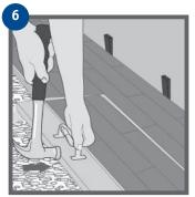
Start the second row of boards with the other part of the cut board. Use Tarkett tapping block to avoid dents. Fully glue the cross joints. Do not glue the others. Joints do not have to be over a batten, but two adjacent rows of boards must never be joined between the same two floor battens.
