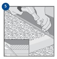
Nail the boards to every floor batten. Hit the nail at an angle (45°) into the angle of the tongue. Use a punch. Do not knock the nail in too far. Use galvanised headed wire nails, dimensions 60-23 mm or a nail/ staple gun. See Nailing section.
