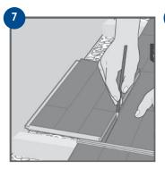
Saw the last row to a suitable width. Lay it (tongue side to the wall) over the next-last row of boards with an approx. 4 mm offset from the wall to give an approx. 10 mm expansion gap when you use an piece of fullwidth off-cut board. Then slide the piece of board along the wall and mark the cutting line with a pencil. If the required expansion gap is wider, offset the final boards by the additional distance necessary. (The tongue of the infill is 6 mm.)
