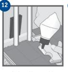
Tap the board into position, glue the loose piece into place, insert a spacer against the wall and cover with pipe sleeve.
