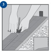
If the last row of boards is narrower than 5 cm or if the wall is not straight, it is advisable to saw the first row of boards. Measure out and mark the cutting line according to the illustration. Check that the row is straight with a guide string.
