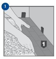
Lay out the first row of boards. Start with the grooved edge against the wall and work towards the right. It is very important that the first row is completely straight.
