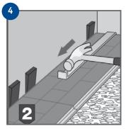
Lay the boards against the wall. Create the required expansion gaps by inserting spacers between board and wall. Glue the end groove of the board you are about to fit. Press it in against the wedges and ensure it lies straight. Tap the joint together using the Tarktool. Hold the board in place with a wedge at the end.
