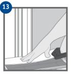
Door linings can be removed and raised, but it is easier to saw them off. Use a spare piece of floor board as a template and saw off the lining with a finetoothed saw. Slide the flooring under the lining. Do not allow the flooring to become wedged tight between the subfloor and lining.
