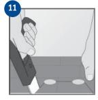
The board's long side meets a pipe: Drill a hole as above. Saw off the piece that will fit behind the pipe, nearest the wall. Cut at an angle as shown in the illustration.
