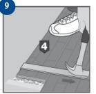
Fully glue the long side's groove side. Tap in the cut board with the aid of the Tarktool. If the last row of boards has not been sawn, the tongue must be sawn off to maintain the expansion gap. Place spacers in the last row of boards as well. Keep the spacers in place for a few hours (e.g. overnight) before they are removed. Note: Do not nail the last boards by the walls. Finish with Tarkett mouldings.
