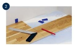
At the end of the row, turn the last board so that tongue lies against tongue. Push the short end tight against the wall. Mark the cut with a pencil, at least 8-10 mm from the short end of the previous board, so that you get an expansion joint when the board is then pushed into place.
