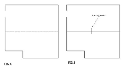
Establish and mark a starting point for the first plank on the center guide line (Figure 5.). When establishing this mark, take into consideration that the first and last plank in each row shall not be less than 8 inches (203mm).
