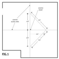
Measure or dry lay a row of tiles from the center point of the guidelines to each side wall to determine the size of the border tiles. If the resulting border is too small, adjust the center guidelines to achieve a larger border tile. When possible, the size of the border tiles shall at least one half the size of a full tile.
