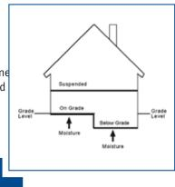
**Below grade** – An acceptable below grade floor is a concrete substrate partially or completely in contact with the ground below the average surrounding grade level. Properly constructed the concrete slab will be suitably protected from moisture penetration by planned water drainage and an installed proven moisture vapor retarder.
