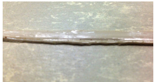
Excessive melting and weld rod breaking are two symptoms of a heat welding gun that is too hot for the pace the operator is moving. The operator will need to increase speed or lower the heat setting.
