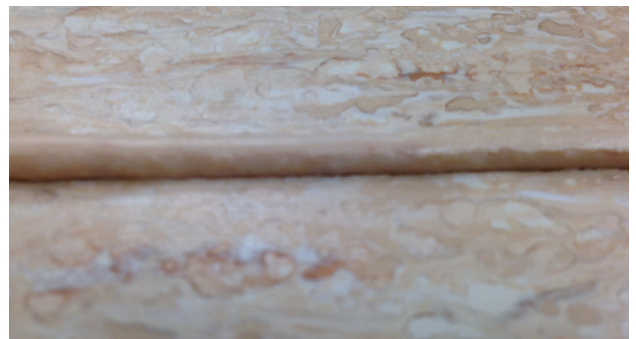
If the rod does not melt it could be a symptom of a heat welding gun that is too cool or the operator is moving too quickly. The operator will need to decrease speed or increase the temperature setting of the heat welding gun.
