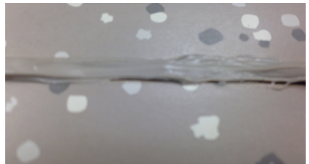
Excessive melting and weld rod breaking are two symptoms of a heat welding gun that is too hot for the pace the operator is moving. The operator will need to increase speed or lower the temperature setting of the heat welding gun.
