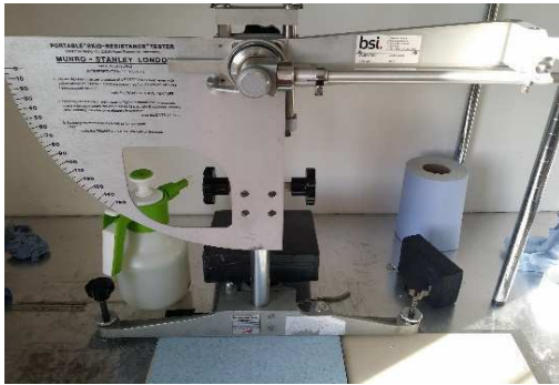
Image 1. Pendulum tester in-situ
