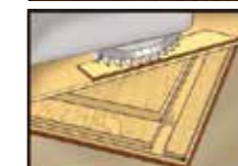
Picture 6: The new board that will be installed, must be prepared first. After you checked the board size, saw off the underside of the short ends and long side, but be careful not to damage top surface and not to remove board tongue.
