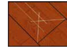
Picture 2: Change of damaged board is done in following way: First cut off the board with circular saw, but be sure that you set the sawing depth max. as thickness of wood flooring (in this case 14 mm). After that saw a "V" from each corner, and then saw from short end to short end to connect these "V" cuts.
