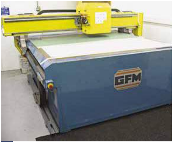
4 Cutting programs are transferred to our sonic cutting machines.
